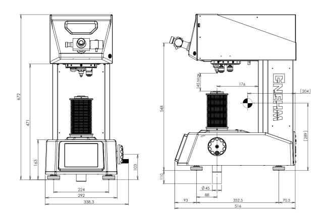
All dimensions in these drawings are approximate and in millimeters. Working heights and workpiece accommodation may vary based on the stages and accessories used.
